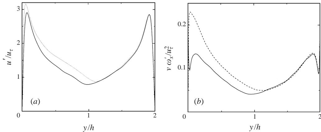
FIGURE 16. (a) Streamwise velocity, and (b) streamwise vorticity fluctuations in: —, a natural channel and ----, the channel in figure 15, in which the boundary condition at the lower wall has been substituted by spanwise free-slip. Normalization is done in wall units corresponding to the natural channel.
