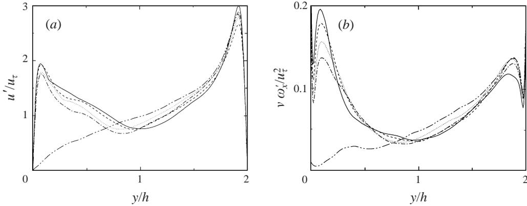
FIGURE 10. Dependence of (a) the streamwise velocity fluctuations, and (b) the streamwise vorticity, for channels with filtered streaks, as a function of filter height: —,  $\delta^+ = 24$ ; - - - , 33; ····· , 44; — · — , 56; — · — · — , 70.
