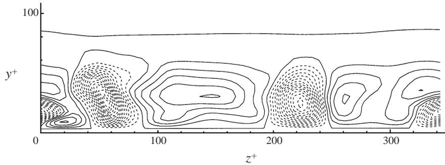
FIGURE 6. Transverse section through the centre of the box in the first frame of figure 5. The streak shown in that figure is the one near  $z^+ = 200$ . Perturbation velocity isolines  $u'^+ = -7.5(0.5)2.5$ . Dashed contours are  $u' < 0$ .
