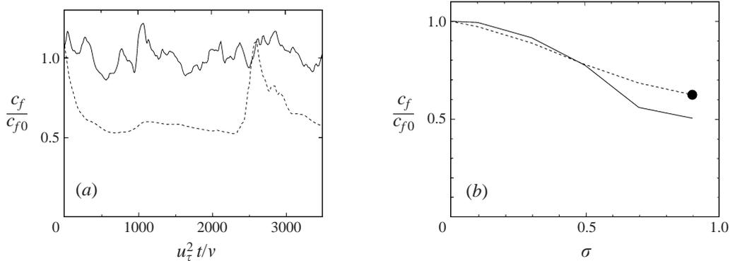
FIGURE 13. (a) Time evolution of the skin friction for a channel in which the source term of the streaks has been filtered with  $\delta^+ = 44$ ,  $\sigma = 0.9$ : —, natural wall; ----, filtered wall. Initial conditions are the same as in figure 9. (b) Reduction in the friction coefficient of the filtered wall with respect to the natural channel, as a function of the filter fraction: ----,  $\delta^+ = 44$ ; —,  $\delta^+ = 85$ . The solid circle corresponds to (a).
