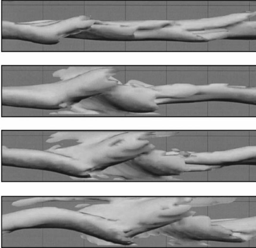
FIGURE 5. Explicitly filtered channel, as in figure 4. The low-velocity streak is visualized as the  $|\omega'|^+ = 0.25$  isosurface of the perturbation vorticity magnitude. The flow is from left to right and the figure looks into the wall. From top to bottom,  $U_0 t/h = 0, 15, 19.5, 25$ . The image is advected with a velocity  $U_c = 0.37 U_0 = 9.7u_\tau$ , to keep the central structure approximately steady. The size of the displayed domain is  $700 \times 115$  wall units.
