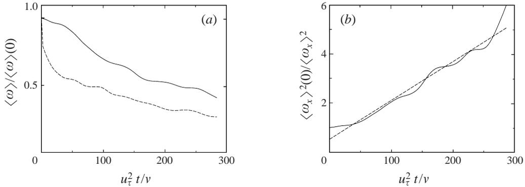
FIGURE 12. (a) Decay of —,  $\langle \omega_x \rangle$ ; and ----,  $\langle \omega_y \rangle$ , in the filtered channel of figure 9. (b) Evolution of  $\langle \omega_x \rangle$ , compared to the prediction for purely viscous decay. The dashed line is (5.5) for  $R^+(0) = 15.8$ . The vorticity norm used is defined in (5.4).
