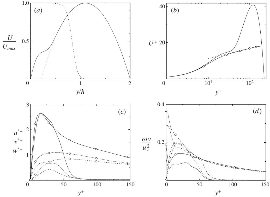
FIGURE 4. Explicitly filtered channel. Lines with symbols correspond in all cases to the full channel by Kim *et al.* (1987). (a) ———, Mean streamwise velocity; ----, filter; ·····, laminar parabola. (b) ———, Mean streamwise velocity in wall units; ----,  $2.5 \log y^+ + 5.5$ . (c) Turbulent velocity fluctuations, in wall units: ———,  $u'$ ; ----,  $v'$ ; ·····,  $w'$ . (d) Turbulent vorticity fluctuations, in wall units: ———,  $\omega'_x$ ; ----,  $\omega'_y$ ; ·····,  $\omega'_z$ .
