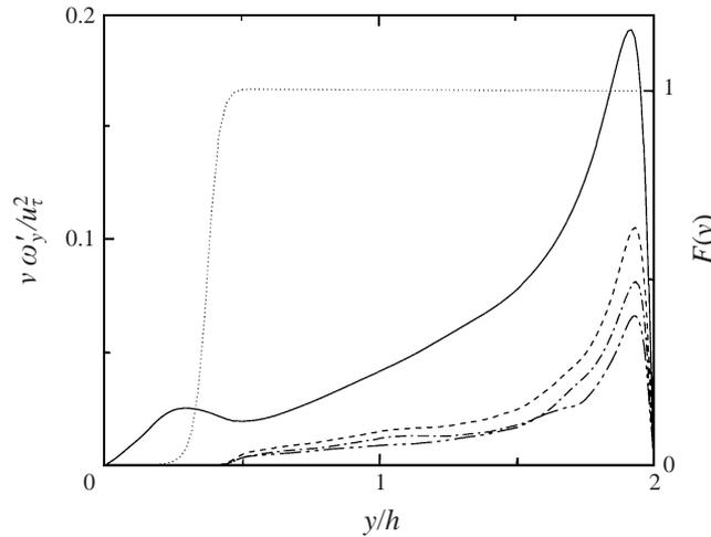
FIGURE 11. Wall-normal vorticity fluctuations for a large channel in which the first two longitudinal Fourier modes of  $\omega_y$  are filtered at one wall.  $\delta^+ = 70$ . —, Full  $\omega_y$ ; — · — , zeroth Fourier mode; — · — · — , first Fourier mode; - - - - , zeroth and first Fourier modes; ····· , filter.
