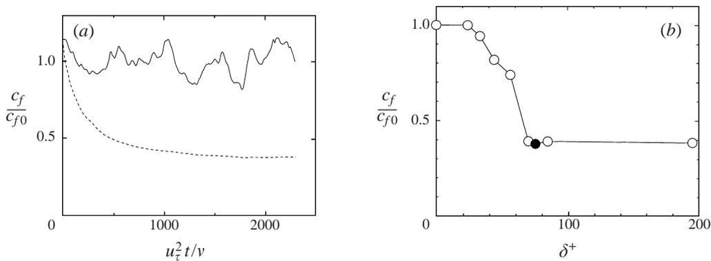
FIGURE 9. (a) Time evolution of the skin friction for a channel in which the streaks have been filtered below  $\delta^+ = 75$ : —, unfiltered wall; ----, filtered wall. Initial conditions are a fully developed channel with  $Re_\tau = 200$ . (b) Reduction in the friction coefficient of the filtered wall with respect to a natural channel, as a function of the filter height. The solid circle corresponds to (a).
