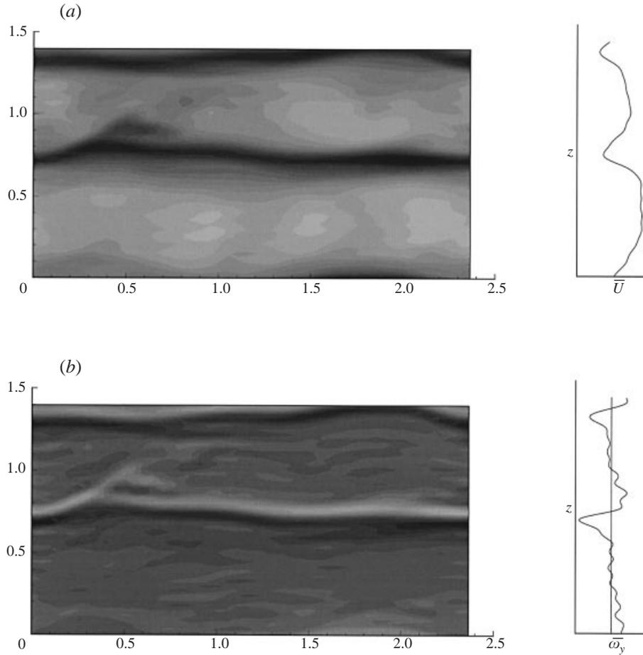
FIGURE 7. Definition of streaks: (a) the streamwise velocity in a plane  $y^+ = 30$ , with its streamwise mean represented on the right; (b) the corresponding normal vorticity. Its streamwise mean value is our definition of ‘streak’. The flow is from left to right, and lighter shades correspond to higher values, as in the grey level scale in figure 8.  $Re_\tau = 190$ .
